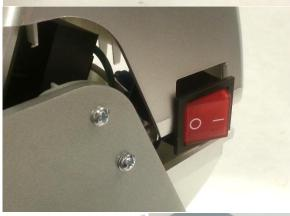
Reassemble Control Housing with Power Switch inserted into slot as shown
