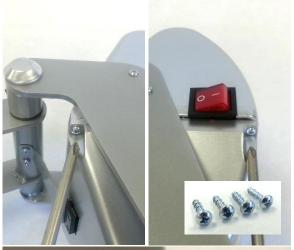
Remove 4x #6 x ½" Screws from control housing using #2 Phillips Screwdriver
