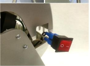
Detach top of Controller Housing and slide old Power Switch out of slot as shown
