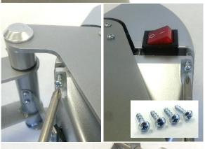
Install top half of Controller Housing and secure by screwing in 4x #6 x ½" Screws using #2 Phillips Screwdriver
