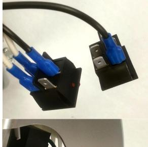
Transfer wires one at a time from old to new Power Switch, carefully matching up terminals
